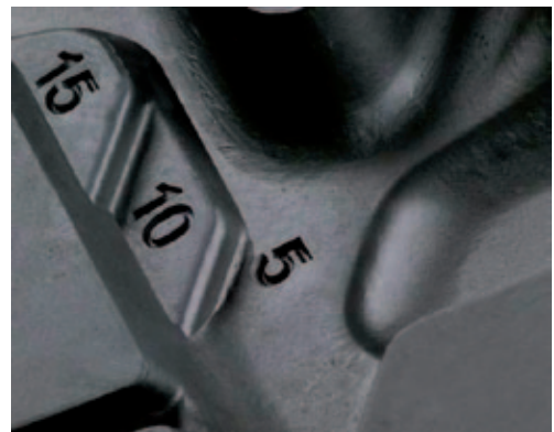
Remaining tread depth in mm 365/80R20 Nokian MPT Agile
